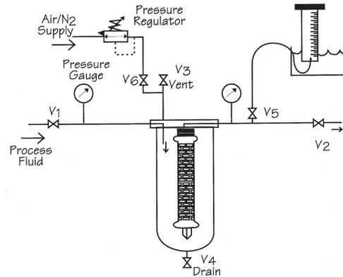
Diagram 3 - Diffusive Flow Integrity Test
