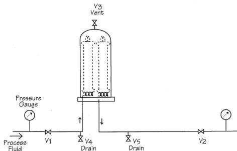
Diagram 2 - Multiple Filter Housing
