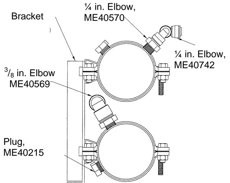
11. Locate the two green product water outlet tubes that are connected to the 1/4 in. elbow fitting (ME40742) on the upper end caps of the membrane housings.
